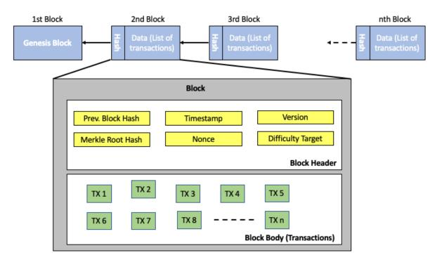
Figure 1: Example of a blockchain containing n blocks, in which each successive block contains the hash of the previous block, a timestamp, the transaction information, the nonce number for the mining process and other details needed for the protocol to work.
